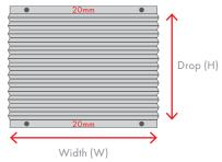
Exclude the 20mm top and bottom fixing and stowage battens from the Drop (H) measurement
