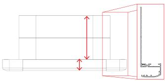
Maximum liner height: 113mm Frame depth: 28.5mm
